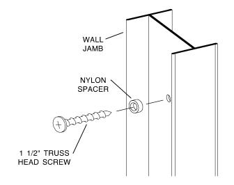
This bath enclosure is equipped with safety tee-lock wall jambs. When properly installed, the header is permanently locked to the wall jambs and cannot be accidentally dislodged.
