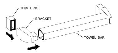
Attach a towel bar assembly (with the open slot in the bar downward) to the interior panel with a #10-24 x 7/8" truss head screw [N] thru the inner rail. Insert a #10-24 x 1 1/8" flat head screw [P] thru an acrylic finger pull [R], thru the outer rail and into the outer towel bar bracket. Peel the backing from a Alumax decal [S] press it into the recess in the acrylic finger pull.
