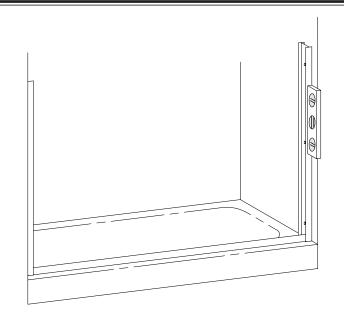
Before replacing the tub track [A], force a slight downward bow in the extrusion. This will ensure the track fits tight to the tub. Run two beads of caulk inside the penciled marks on the tub rim. Place the tub track in the exact position marked in Step #2 and seat it firmly in the caulking. NOTE: Improper caulking will result in leaks.
